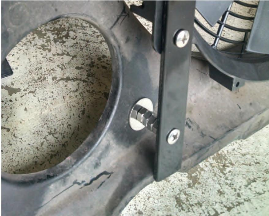
4. For this corner I just made a standoff by stacking 5 nuts for the appropriate height and attached to the shroud at an available spot. I used fender washers to reinforce the shroud at the attachment point. The screw at this corner is 2" long, the others are all 1" long.
