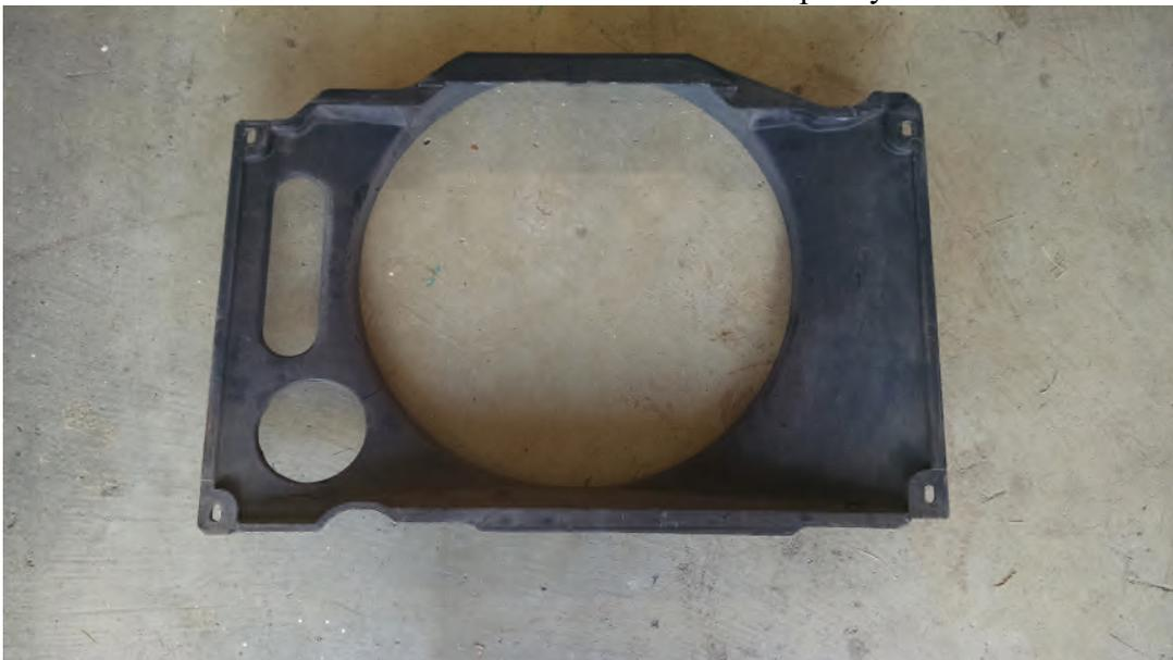
2. Remove fan shroud (if not already removed from radiator)
