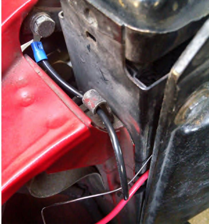
7. A chassis bolt near the upper left corner of the radiator makes a convenient ground attachment point. For a power supply, I ran a heavy gauge wire with an inline fuse directly to the (+) battery terminal. This is simpler than finding a good supply point downstream of the ignition switch. It means that the fan continues to cycle according to coolant temperature after the engine is shut off, which I don't mind.
