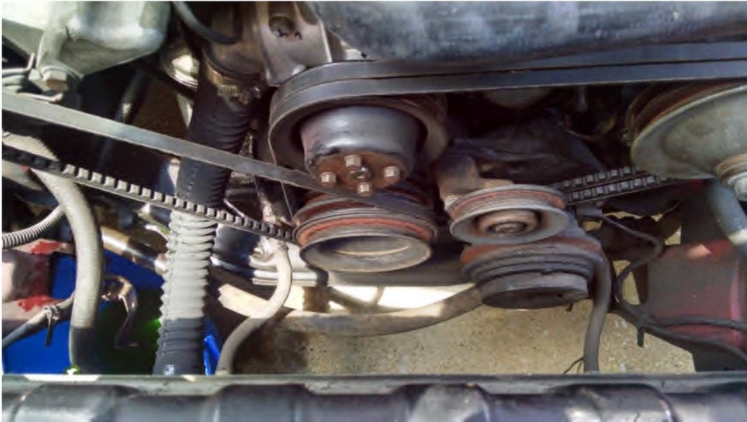
1. Remove stock fan and reassemble V-belt pulley without fan.
