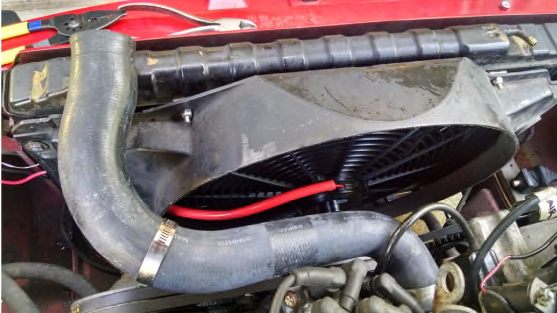
5. Insert the temperature probe from the switch through the fins of the radiator near the upper radiator hose outlet. Reinstall the shroud with the fan attached, with the wiring extending between the radiator and the shroud at the left hand side. The thin silver wire shown here is from the temperature probe, the red and black wires are power to the fan.
