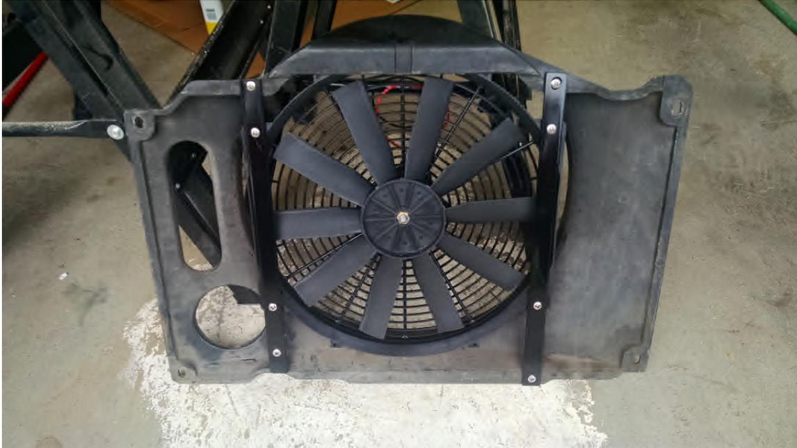
3. Cut aluminum bars to fit shroud and drill holes to match fan mounting holes and to fit convenient locations on shroud. Note that lower end of RH bar (shown at left in this view) is cut away to clear radiator hose and has no flat mounting surface available.
